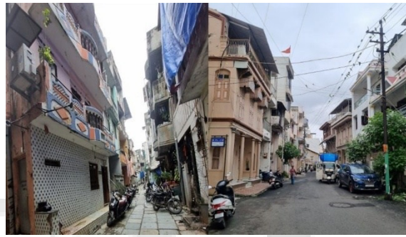
Figure 16 Airflow Obstruction Left: Nanpura's narrow lanes flanked by tall, closely packed buildings restrict cross-ventilation, contributing to indoor heat stress. Right: Rander's dead-ended, labyrinthine alleys further limit air movement, amplifying discomfort during humid and monsoon conditions.
