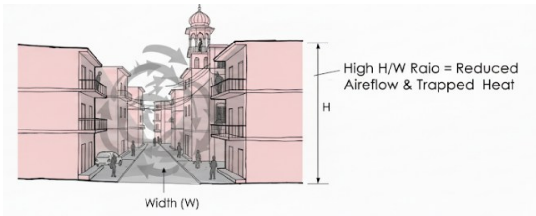
Figure 26 Street canyon section illustrating how a high height-to-width (H/W) ratio restricts airflow and traps heat, reducing thermal comfort in dense urban corridors.
