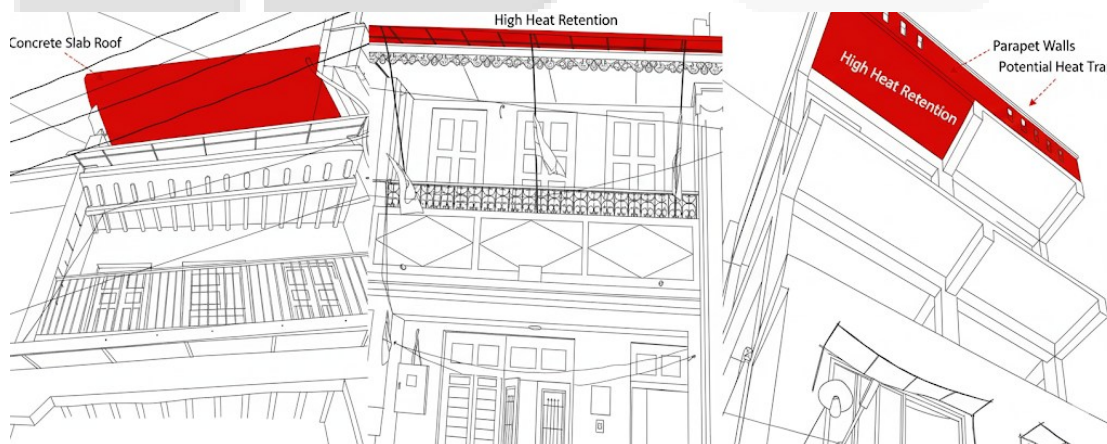
Figure 13 Annotated rooftop heat retention analysis: Comparative sketches highlight thermal vulnerabilities in concrete slab roofs, flat terraces, and parapet-walled structures—each marked in red to indicate zones of high heat retention and potential thermal discomfort.
